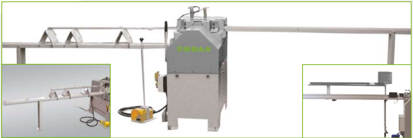
GLS 102 with measuring feeler 1.5 m and profile support 3 m (also available with 6 m). Small picture, left side: measuring feeler 3 m. Small picture, right side: servo-length stop.
